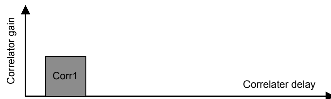
Figure 3.4: An example of indoor channel and RAKE receiver finger delay
